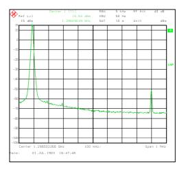
We can see spurious in the output spectrum. The level is lower than specifications ( < -60dBc).
