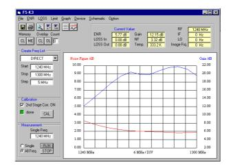
I must work on the first stage to improve the NF result. The goal is better than 1.5dB.
